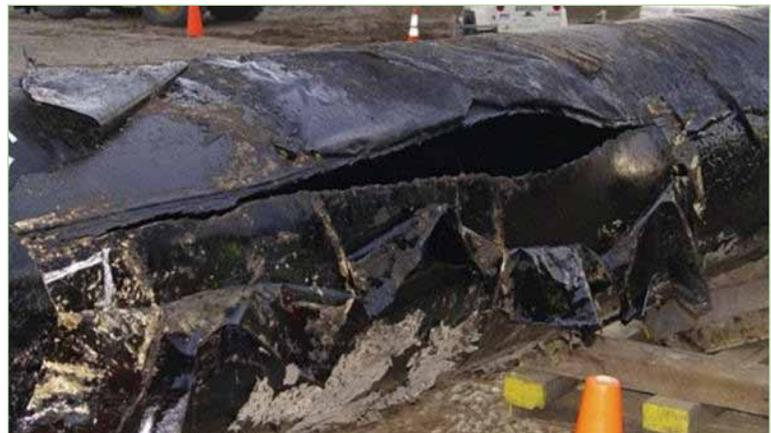
*The Enbridge pipeline that failed in Michigan in 2010 had older enamel wrap coating installed*
