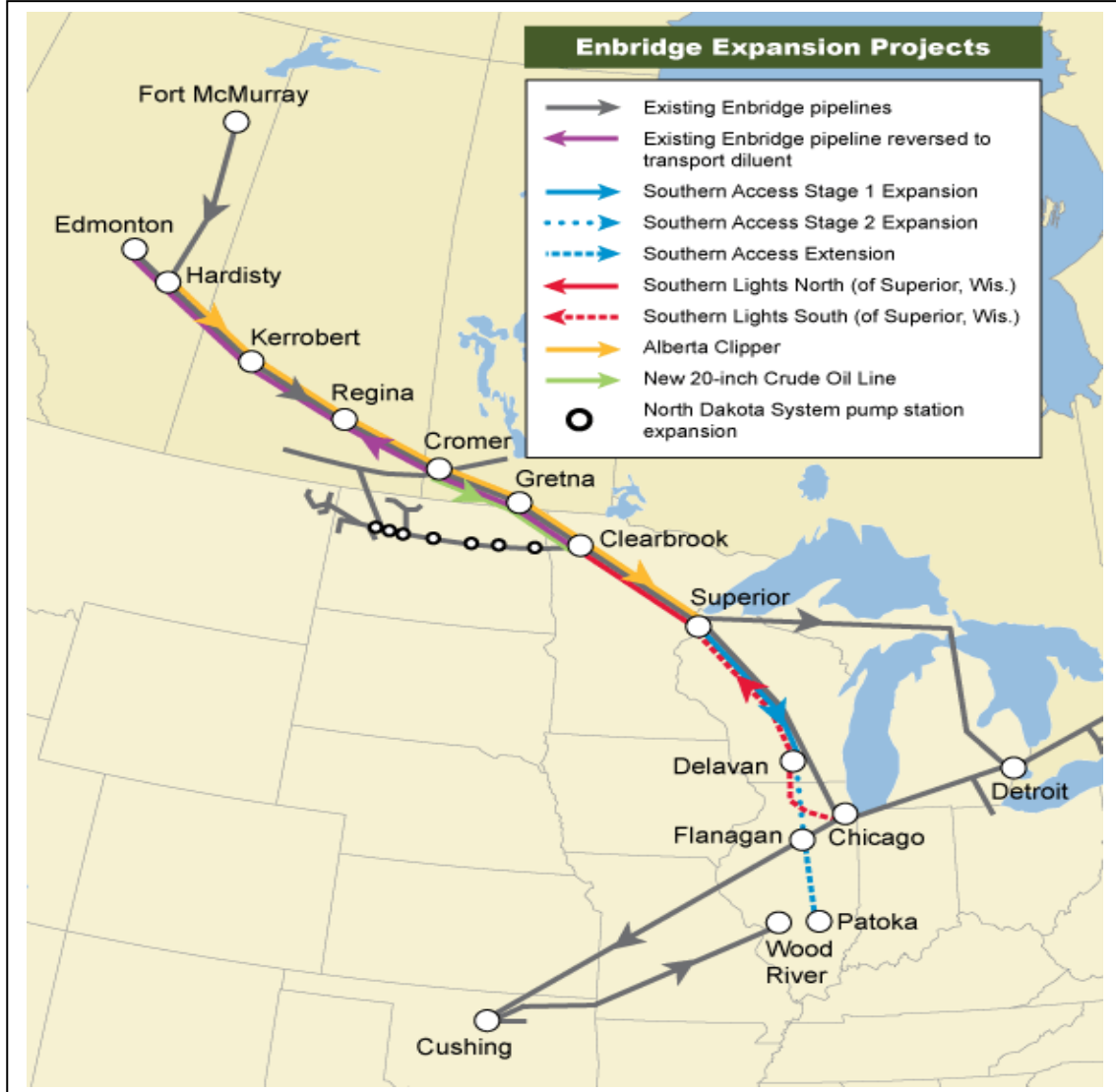
Figure 2: Enbridge Pipeline Expansion
